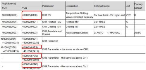
Enter the settings by each channel after checking the address.
