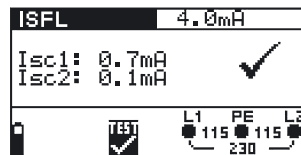
Figure 11.6: Example of a first fault current measuring result
