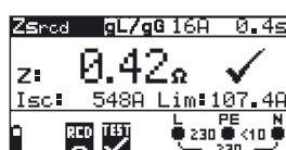
Fig. 5.32: Example of loop impedance measurement results
