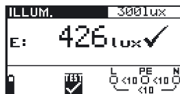
Fig. 5.52: Example of illumination measurement result
