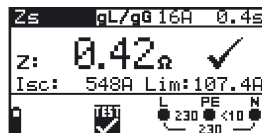
Fig. 5.30: Example of loop impedance measurement results
