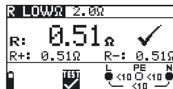
Fig. 5.8: Example of LowΩ resistance measurement results
